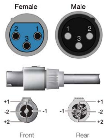
Figure 5. Cannon® XLR and Neutrik® SpeakOn connectors
